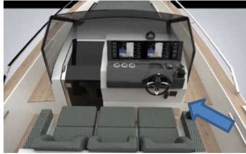
FIG. 4.5-1 - manual activation of the fire extinguishing system
